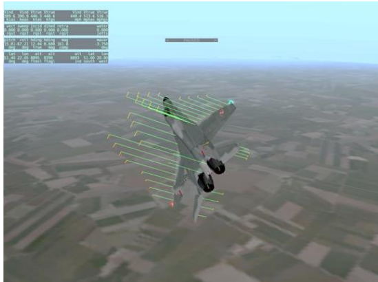
Figure 2: Example of screen from X-plane software (lifting force).
