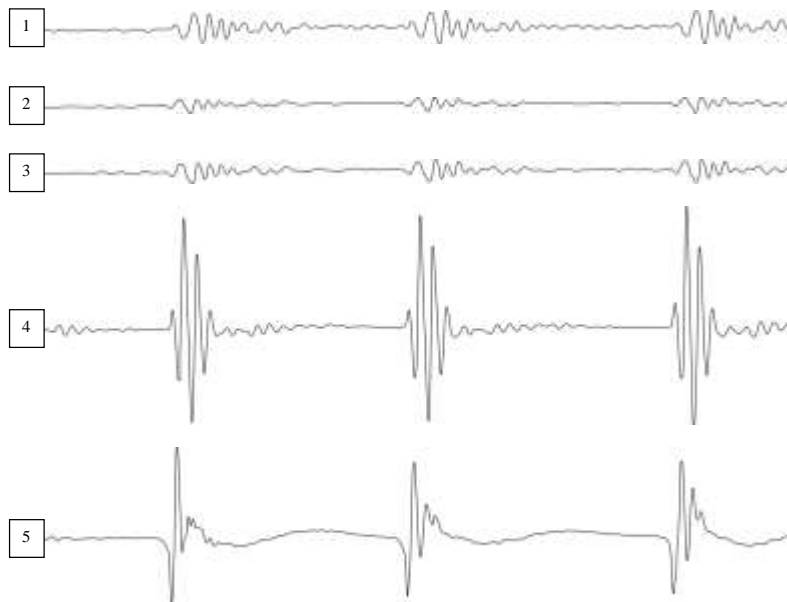
Fig. 4. Digitized record, pile no. 2, depth of 4 m, vertical component
