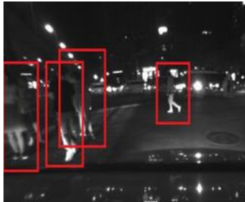
Figure 8. Identification of pedestrians
